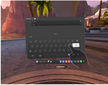
Fig. 1. Virtual interface from the victim’s perspective. The user performs mid-air typing on a standard QWERTY keyboard, with a hand silhouette (bare-hand tracking) pointing to select keys.
